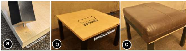
Figure 9: Fabrication of a stool using an AccelLumber panel. (a) Attach the stool legs by fastening them into the pre-drilled pilot holes in the AccelLumber panel. (b) The finished stool, without a cushion. The dashed box indicates the location of the electronic components embedded within the panel. (c) The stool with a cushion placed on top, which does not obstruct the RF energy emitted from below.
