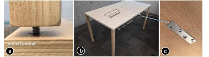
Figure 7: Fabrication of a desk using AccelLumber panels. (a) Attach the legs by screwing them into pre-drilled pilot holes within an AccelLumber panel. (b) The completed desk assembly. The dashed box indicates the location of the electronic components (power management, BLE, MCU, and accelerometer) embedded within the panel. (c) The desktop was constructed using two AccelLumber panels joined with flat brace brackets.
