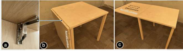
Figure 8: Fabrication of a drop-leaf table Using AccelLumber panels. (a) The drop leaf was attached to the tabletop with self-supporting hinges. (b) In the folded position, the drop leaf rests downward. (c) When lifted, the leaf extends to create a larger flat surface. The AccelLumber is capable of detecting the open and close motion of the drop leaf. The dashed box indicates the location of the electronics components embedded within the panel.
